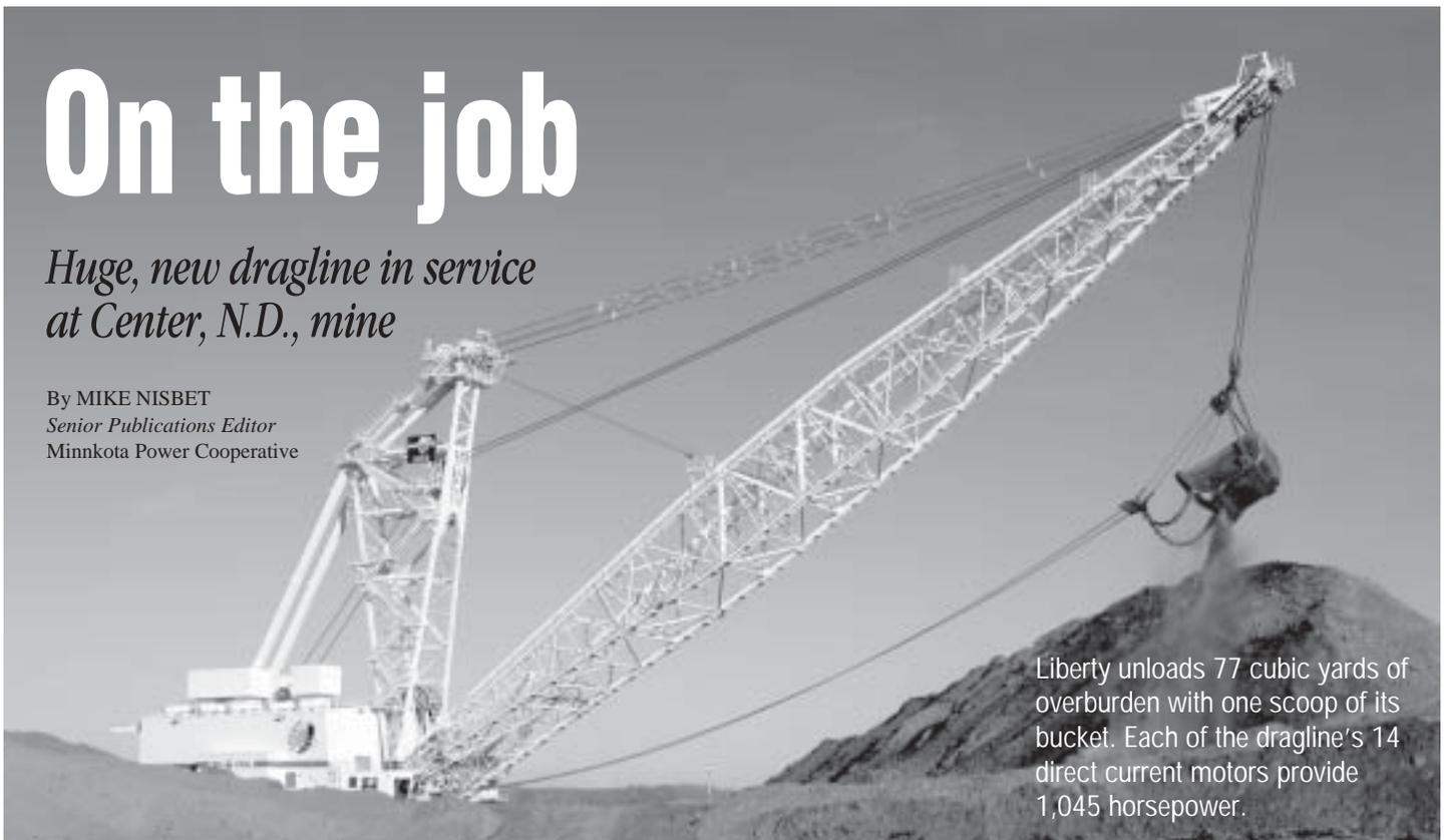
Liberty unloads 77 cubic yards of overburden with one scoop of its bucket. Each of the dragline's 14 direct current motors provide 1,045 horsepower.
